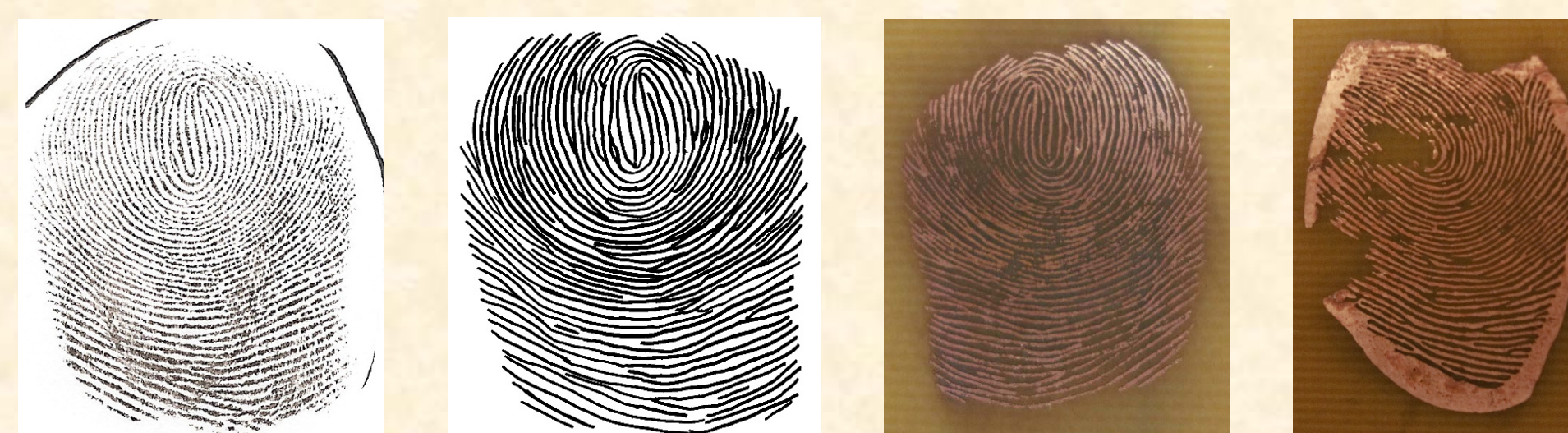
Figure 3: (L-R) (1) Raw print captured with stamp ink pad, then traced by hand to produce image (2). (3) Negative mold of print in image (2) produced via the printed circuit board method. (4) Negative mold of print that was enhanced in Figure 3 via the printed circuit board method.
